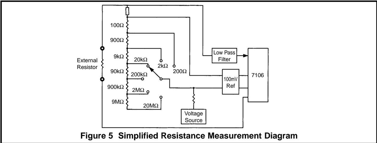
Figure 5 Simplified Resistance Measurement Diagram
