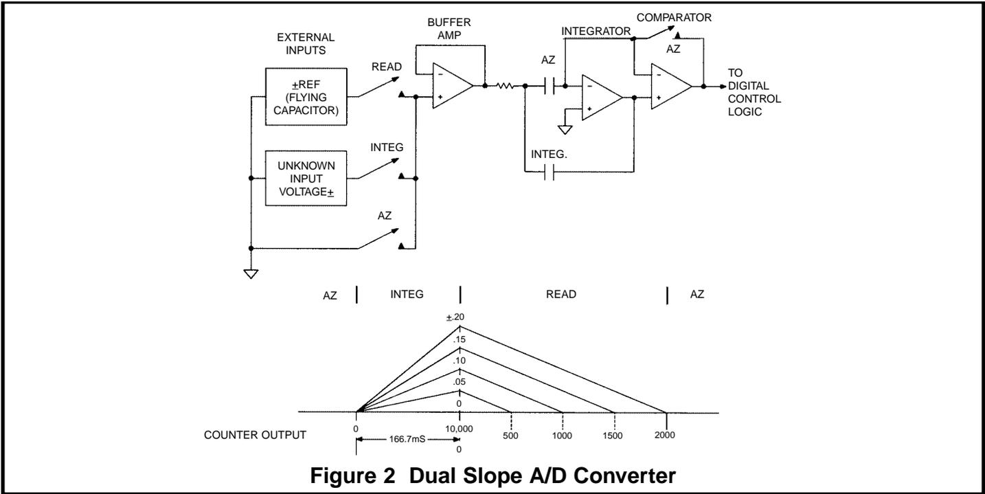
**Figure 2 Dual Slope A/D Converter**
